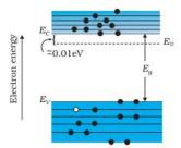
The semiconductor obtained is N-type semiconductor and the majority charge carriers are electrons.
