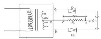
Change the connection of R from point C to point B. Now No Current flowing through D2 in the second half.
